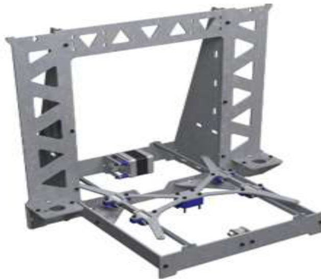
Fig. 6: FreeCAD model of the designed 3D printer frame.
