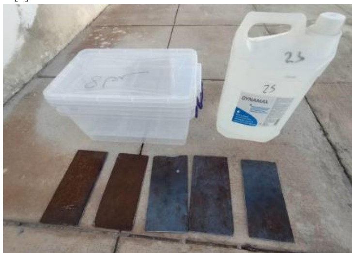
Figure 3.3: Steel samples after cleaning and standardized surface preparation.
