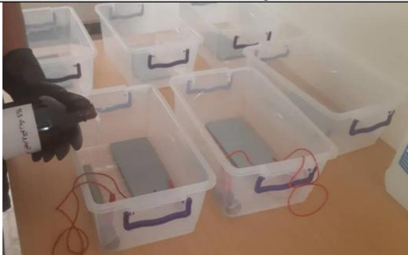
Figure 3.4: Samples immersed in test solutions during the four-week exposure period.
