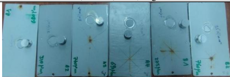
Figure 3.2: Complementary view of the prepared steel substrates.
