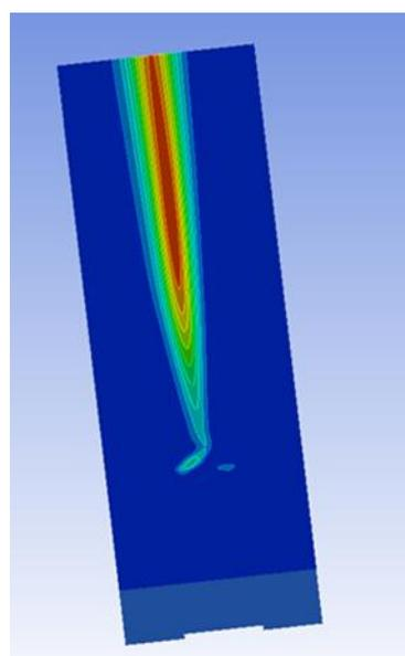
Figure 15: Gas concentration at the second level of the Model One.
